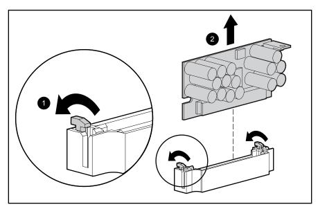
Figure 2-32. Removing the processor power module.
